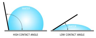
An optimized DWR keeps droplets in a rounder shape—like a dome-shaped bead. The rounder the droplet, the easier it rolls off the fabric. A low contact angle permits droplets to assume a flatter shape, one that can spread out like a splotch, cling to the fabric's surface and eventually seep into it.
